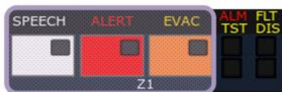
Figure 5-4 Emergency zone with controls highlighted
