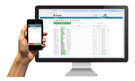
Nimbus is a non-intrusive add-on to the Ampac FireFinder and FireFinderPLUS range of control panels and communicates to a cloud hosted database using the Nimbus Dual Path Gateway.
