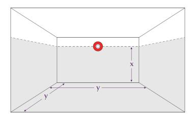
X – The maximum height of the device on the wall in metre: with a maximum value of 2.4m.
