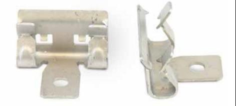
Beam clips may be used to support the LHD cable directly (in this case a separate silicon pad is required) or fixed to other mounting brackets and used to affix the bracket to a RSJ/l-beam or equivalent.
