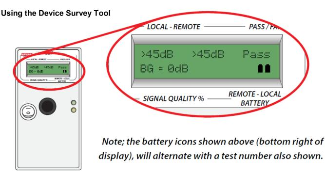
With the Device Survey Tool switched on, depress the rear switch to initiate a signal. After a few seconds results will be displayed and a high pass or a at fail tone will be heard.
