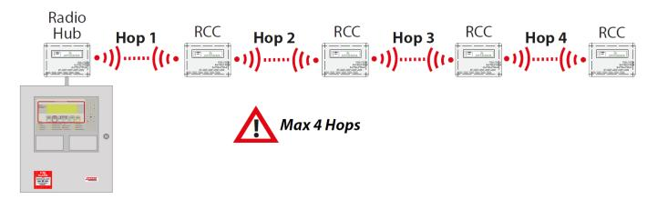
5. Remember, the RCCs can each accommodate a maximum of 31 wireless devices.
