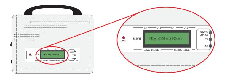
Once switched on, the Signal Surveyor's display will show the current background interference level. To achieve the maximum signal distance the background level should be as low as possible. This level is shown between 000 and 100. If the background levels are high, try repositioning the unit. Then turn off and back on again. This will re-show the background level for the new position.
