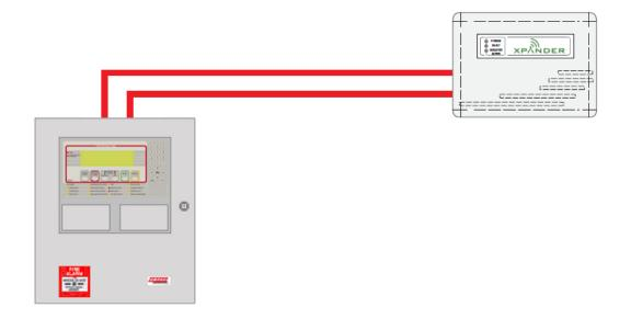
2. Remember when choosing a location, the Diversity modules require a loop in and out cable connection and a maximum of five RLMs per loop are allowed.
