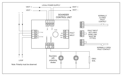
Fuse: 1.0A, anti-surge Local supply: 24V (9—32V) Sounder zone end-of-line resistor: 10KΩ, ½ Watt
